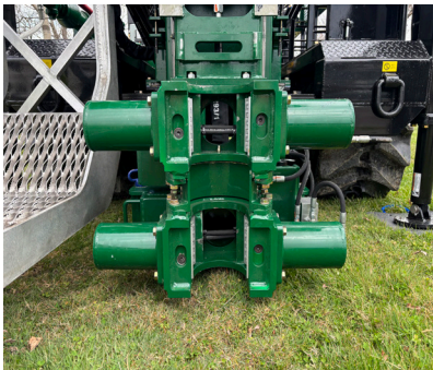
All - New Hydraulic Double Rod Clamp System, featuring articulating top jaws
