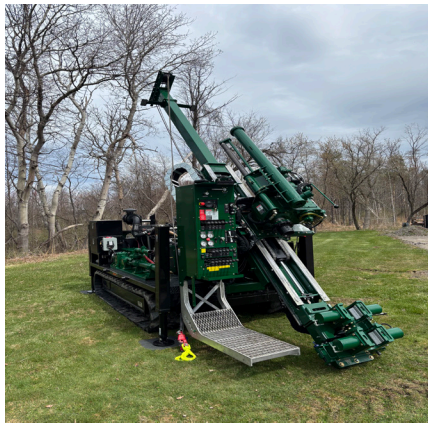
Lockable Mast Brackets work in conjunction with the dump mast to allow for premier angle drilling capabilities.
