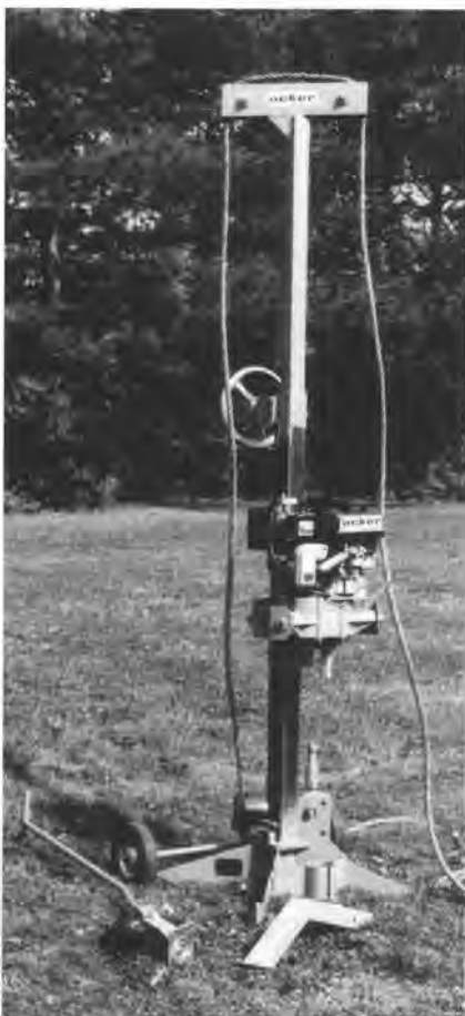
Standard Model "S" Soil Mechanic for auger drilling soils. Note: Hand feed wheel, auger power head and drill platform. Ideal for shallow investigations. Cathead Optional.
