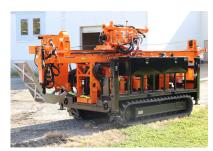
The REBEL XL is a midsize, all-hydraulic, multi-purpose drill rig. It's design and power make it proficient for augering, coring, and SPT.
