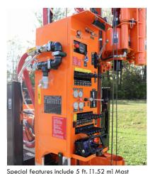
Dump for convenient positioning when angle drilling or drilling on uneven terrain, Engine Tilt for drilling on hillsides up to 45 degrees, Dual Action Slide Base, dual Water Pump configurations, lighting packages, etc.
