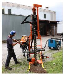
Feed system allows 77" [195.5 cm] stroke for standard applications, or 44" [111.7 cm] stroke for low clearance applications. Low clearance mode allows for drilling under 8 ft. [2.4 m] clearance.
