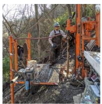
In addition to the "high torque" Auger Drill Head rated at 1,014 ft. lbs. [1,372 Nm] of torque, the Kodiak also includes a "high speed" Coring Drill Head rated at 577 RPM. Optional Wireline Hoist available upon request.
