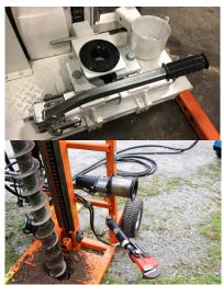
KODIAK includes Cathead, Rod Clamp, Hydraulic Breakout Wrench, Auger Guide, and Rod Bushing.
