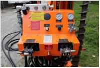
Feed Speed, Feed Pressure, Rotation Speed, Cathead, and Optional Wireline Hoist are all easily adjustable from the Control Panel.
